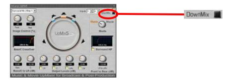
This push button applies a stereo downmix to the 5.1 processed ouput signal. It corresponds to the downmix described by the ITU (ITU-R BS.775) with the specific BBC Research Department recommendation:
