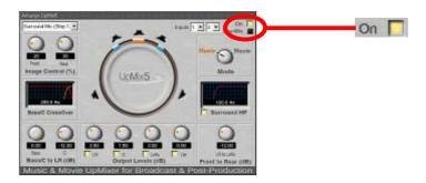
The *On/Off* push button allows user to activate or deactivate the upmixing process in order to compare with original material. The signal is always routed through the plugin in both On and Off positions. Thus, there is no latency difference between the two states (activated and deactivated).
