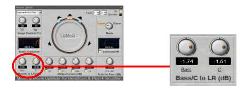
Thus, two divergence controls allow user to control the amount of C and bass signals sent to the front LR channels. Both divergences are applied after the CrossOver filter. The amount of C in LR is dynamically shown on the surround circle with the yellow figure.
