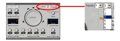
The *Inputs Selection* list show which input channels are selected. The first list represents the Left channel and the second list the right channel of the stereo input. The inputs 1 and 3 are the default stereo inputs.
