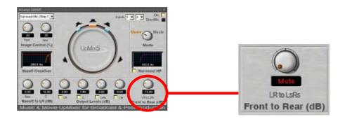
A part of the extracted stereo component can be routed to the rear channels allowing a more accurate enhancement effect. The *Front to Rear Divergence* is applied before the center divergence to LR and before the surround High Pass filter. Therefore, any bass or mono central component can be sent to the surround speakers. The amount of LR in LsRs is dynamically shown on the surround circle with the green figure.
