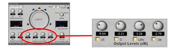
A 5.1 balance allows user to control front L/R, center, surrounds and subwoofer output levels. Each level can be muted by deactivating the corresponding push button.
