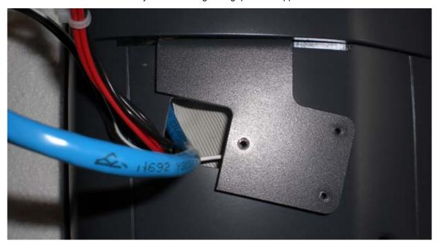
Attach each support using three M3 X 6mm screws, washers and star washers. Be careful to ensure that the cables are not pinched under the support.
