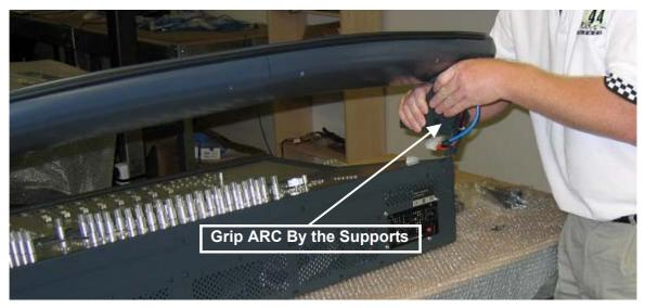
Once the **ARC** is aligned, carefully lower it into position and continue to support it while the fixing screws are inserted and tightened.
