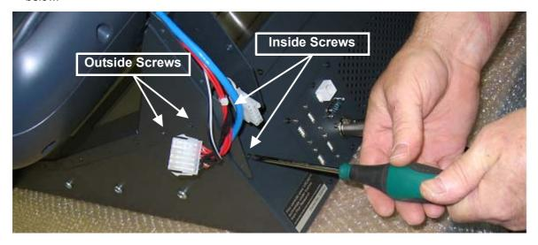
When all the screws are in place, tighten each of them. Repeat this step for both sides of the console.
