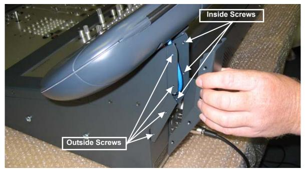
When all the screws are inserted, tighten each of them.
