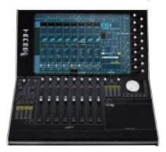
he Smart Console introduced the concept of the 'ARC' touch-sensitive display that offers rapid access to a large number of channels and enables parameters to be applied to multiple channels quickly. The first Tango took the concept further by applying it to the top of a large touchscreen where a wipe across the top enables you to scroll across 240 channels and gives almost instant access to any channel. Tango 2 takes the game to another level with its enhanced user interface.
